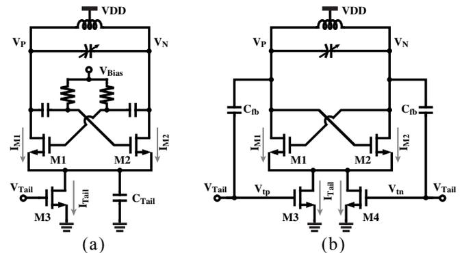
Fig.1. (a) Class-C VCO and (b) tail-current modulated VCO.
