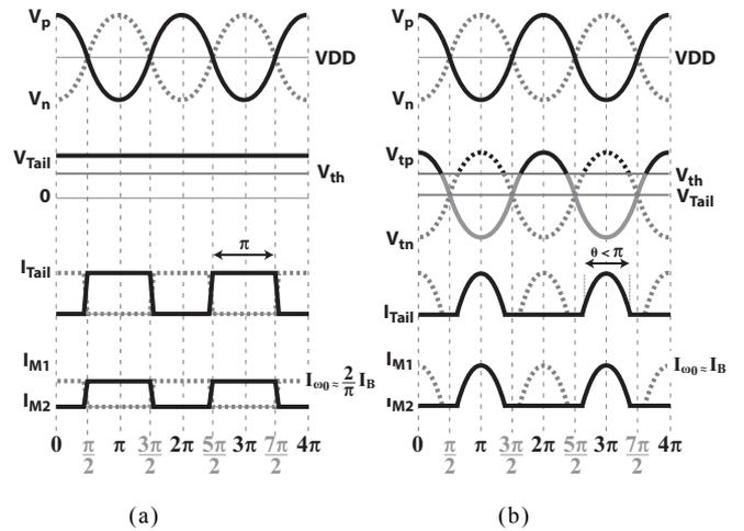
Fig.2. (a) Waveforms of interest in class-B and (b) tail-current modulated VCO.
