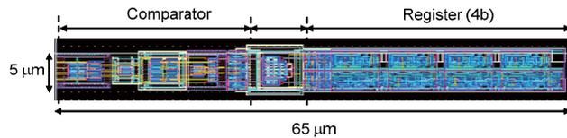
Fig. 7. Layout of the double-tail latched comparator.
