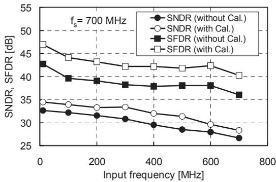
Fig. 11. SFDR and SNDR vs. input frequency.
