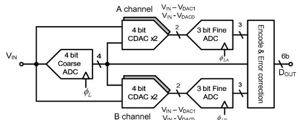
Fig. 1. Proposed subranging ADC architecture.
