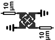
◆Additional 10 µm transmission lines to be deembedded
