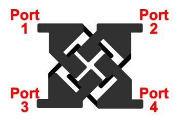
$$S_{CCC} = \begin{bmatrix} S_{11} & S_{12} & S_{13} & S_{14} \\ S_{12} & S_{11} & S_{14} & S_{13} \\ S_{13} & S_{14} & S_{11} & S_{12} \\ S_{14} & S_{13} & S_{12} & S_{11} \end{bmatrix}$$
