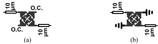
Fig. 3. Remaining responses after de-embedding and solving for one structure (a) cross-line terminated ports with open circuit, and (b) cross-line terminated ports with short circuit.
