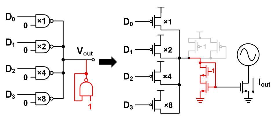
A feedback structure for forming a current mirror.
