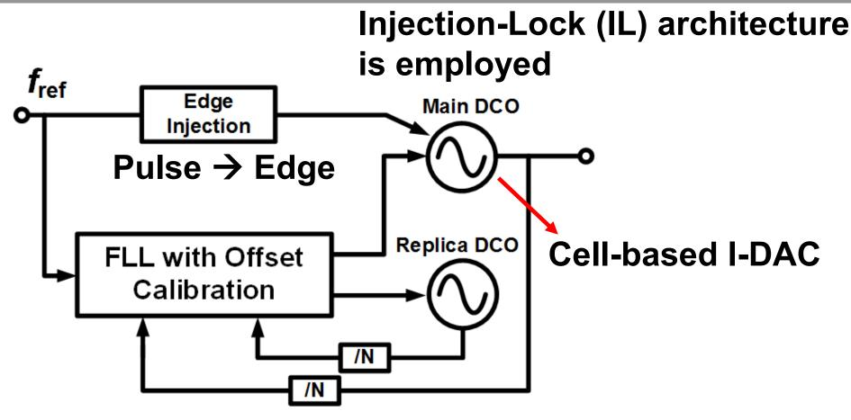
Feedback FLL for frequency tracking Feedforward edge injection for phase locking
