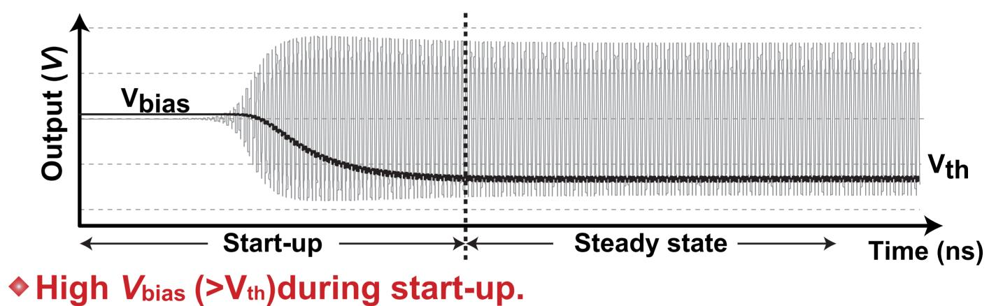
◆ *V*<sub>bias</sub> is gradually reduced for optimum enhancing efficiency.
