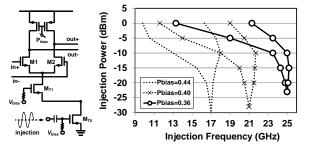
Fig.2 Asymmetrical locking range caused by large injection amplitude in an ILFD proposed in (2)
