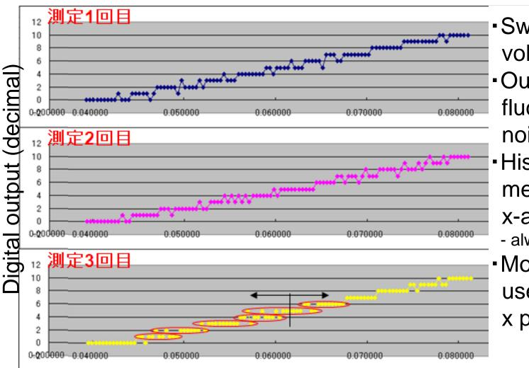
Sweep input voltage by ramp Outputs fluctuate by noise Histogram method ignores x-axis positions - always monotonic Moment method uses averaged
