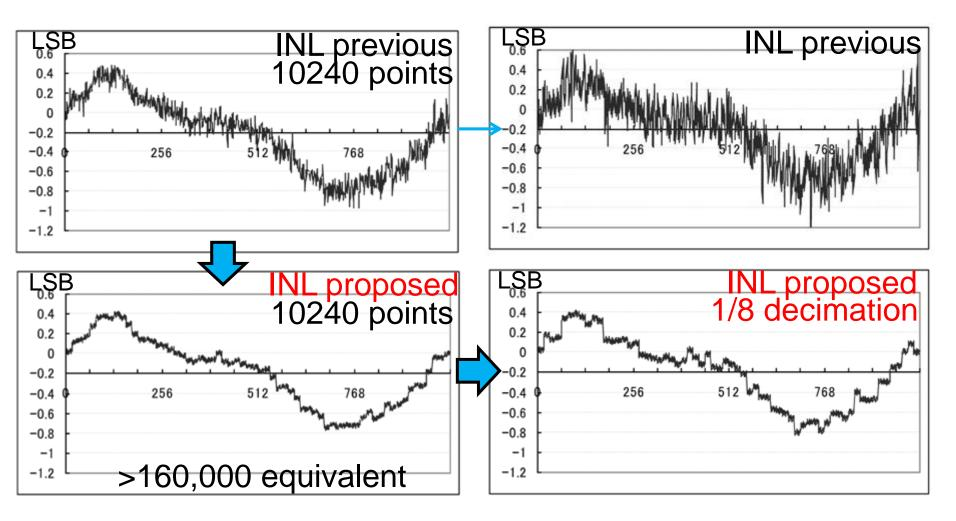
Novel Measuring-Noise-Suppression and Measurement-Time-Reduction Methodology for ADC/DAC
