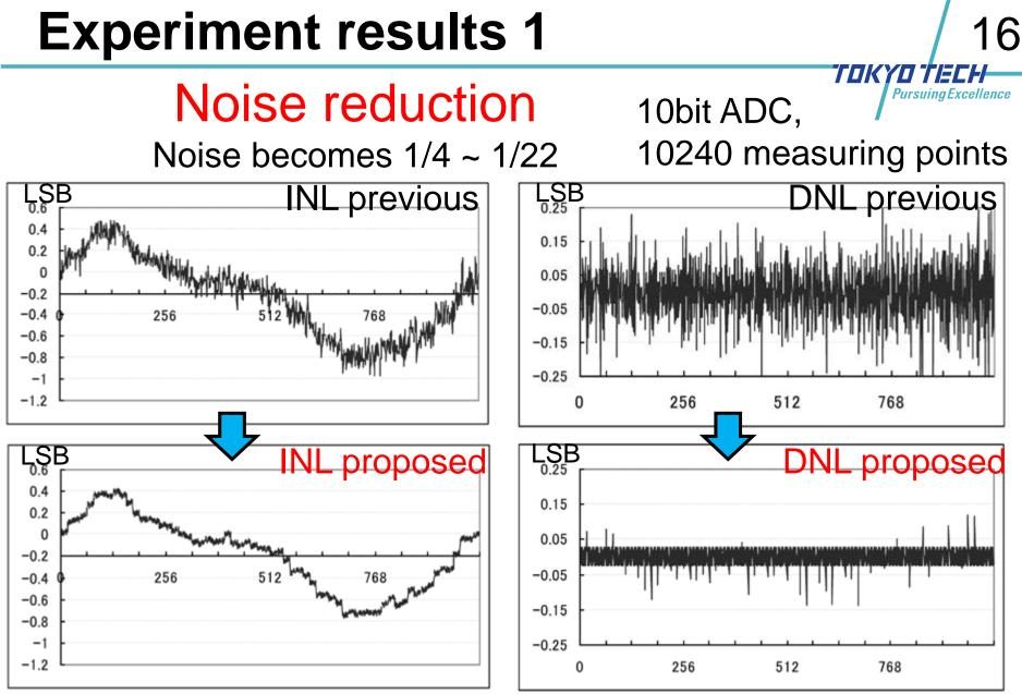
(Equivalence of x16 = 160,000 measuring points or more) Novel Measuring-Noise-Suppression and
