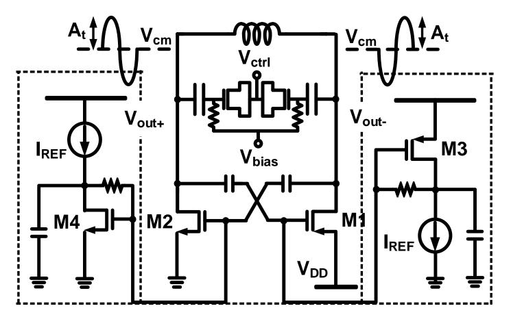
Dynamic Bias Control Circuits for Class-C operation
