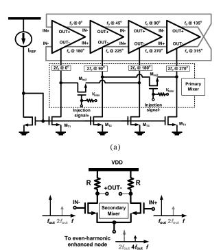
(b) Fig.3. Detailed circuit schematic of the proposed (a) dual-step-mixing ILFD and (b) its delay cell
