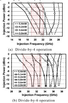
Fig.5. Measured locking range of the proposed ILFD
