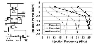
Fig.2 Asymmetrical locking range caused by large injection amplitude in an ILFD proposed in (2)
