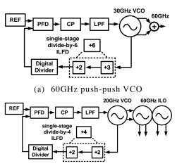
(b) Sub-harmonic injection based on 20GHz PLL Fig.1. 60GHz frequency synthesizers proposed in [1],[2]
