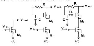
Fig. 1 (a) CS topology, (b) cascode topology, (c) Gain-boost cascode topology.
