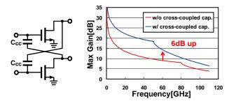
Fig. 4. Negative capacitance and the maximum gain.
