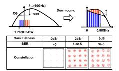
Fig. 5. Gain flatness and the constellation for the 16 QAM.
