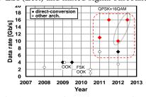
Fig. 3. Data rate in 60 GHz transceivers.
