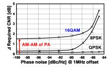
Fig. 6. Requirements for the phase noise.
