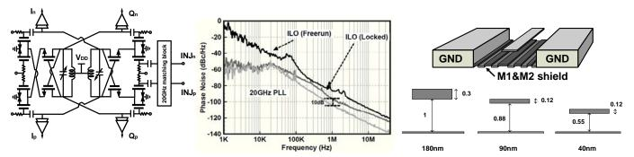
Fig. 7. Injection locked 60 GHz I/Q VCO and phase noise.
