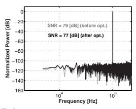
Fig 3 Noise increase caused by settling time optimization
