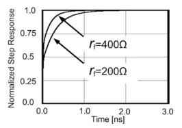
Fig 2 Step response of the single-stage amplifier
