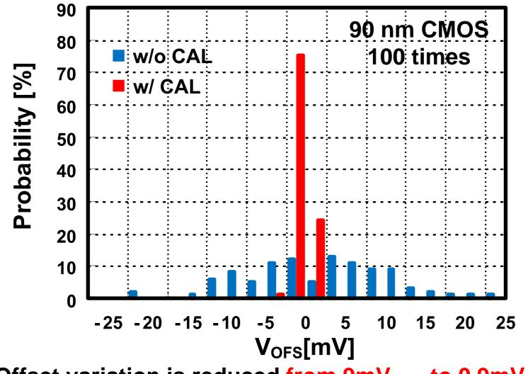
Offset variation is reduced from  $9mV_{RMS}$  to  $0.9mV_{RMS}$ .
