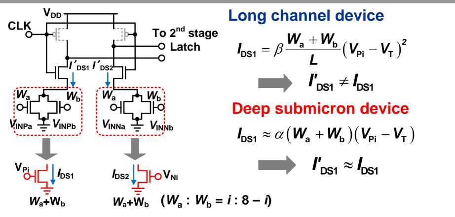
Advantage : Power consumption increases very little. Disadvantage : Interpolation error because of non-linear characteristic of MOS FET.
