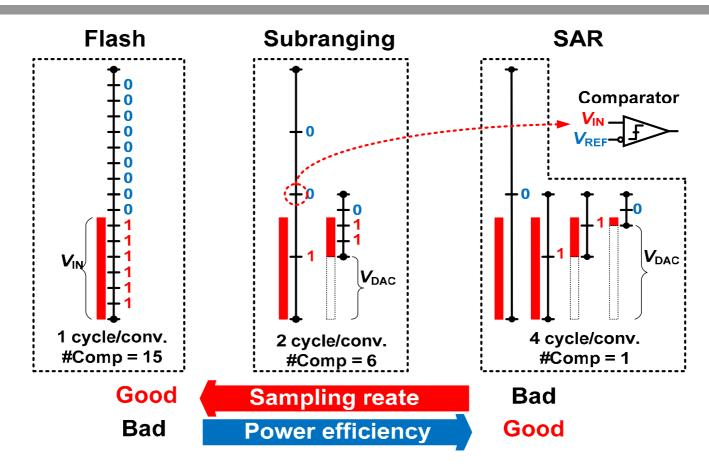
6~7bit, around 1GS/s operation Flash → Poor power efficiency SAR → Extremely high speed CLK (6GHz~) Subranging → Good balance
