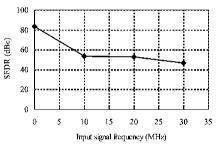
Fig. 1: SFDR versus input signal frequency,  $f_{samp} = 100$  MHz (taken from [2]).
