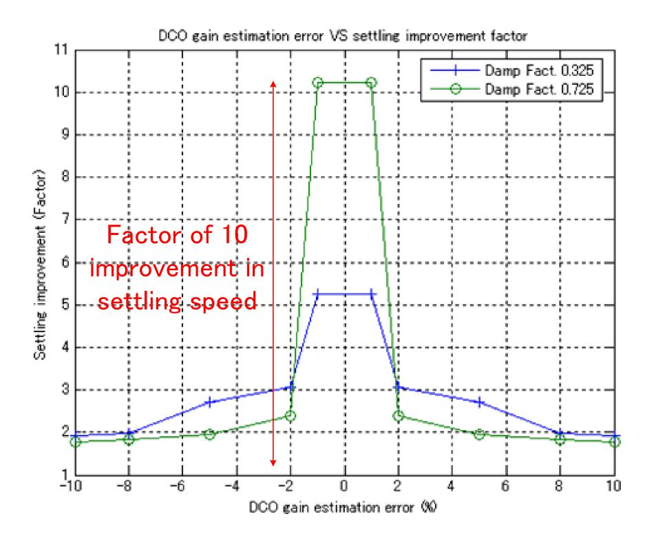
Fig. 5: All Digital Phase-Locked Loop Settling time improvement VS DCO gain estimation error
