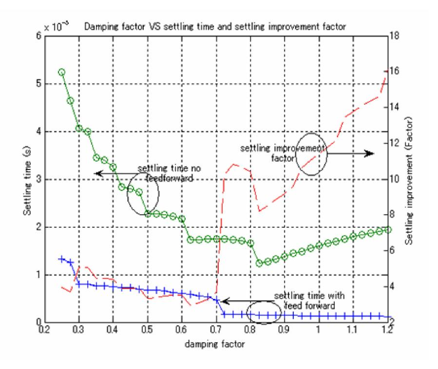
Fig. 6: All Digital Phase-Locked Loop Settling time and improvement factor VS damping factor at 1% DCO gain prediction error
