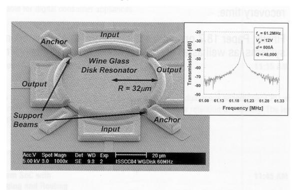
Fo=61MHz Q=48,000 -145dBc/Hz far-end -115dBc/Hz @ 1KHz
