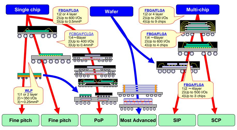
Remarks: 1) Necessary substrate layers, 2) Existing pin count, 3) Terminal pitch
