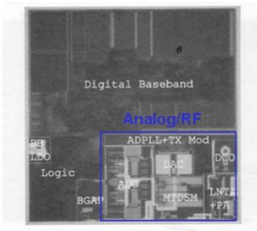
jure 15.1.7: Die micrograph of the single-chip Bluetooth transceiver.
